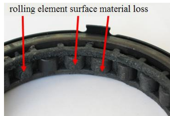
Fig. 8. Effect of sliding operation on the bearing rolling elements
