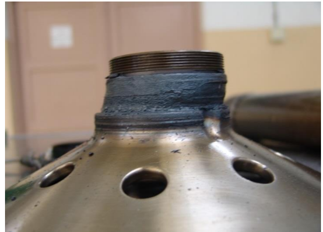
Fig. 7. Plasticized bearing journal
