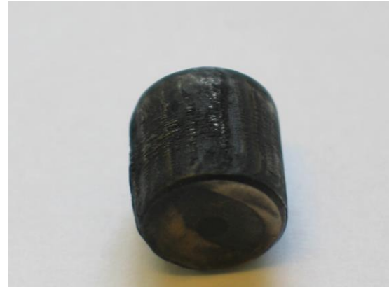
Fig. 10. A rolling element of a bearing with too large interference fit; signs of 'milling' and surface waviness due to heat-induced wear-and-tear are evident
