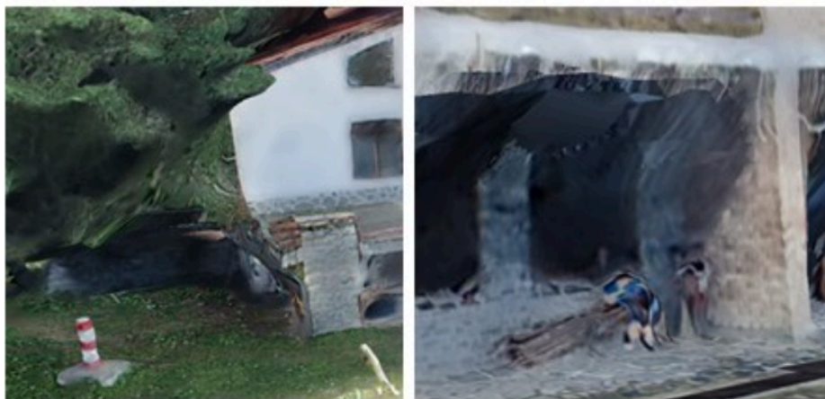
Fig. 11. Disadvantages of 3D models obtained by aerial photography with a UAV
