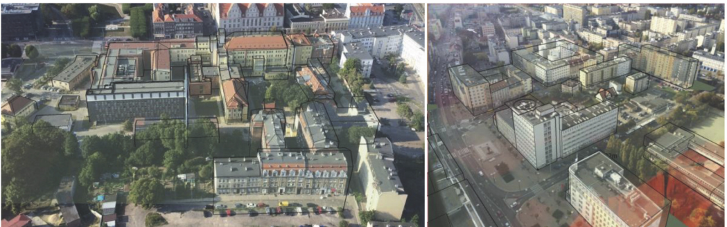
Fig. 3. Usage of photogrammetric technique to obtain geometry of surrounding buildings from aerial photography [based on Helitech, 2014]
