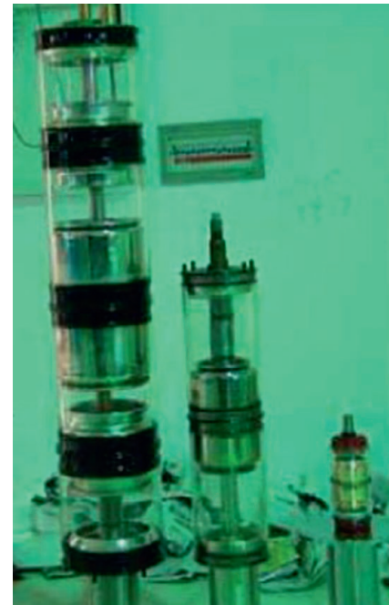
Photo 1. Comparison of vacuum chambers in circuit breakers for highest, high, and medium voltages (from left) 245, 126 and 12 kV [6]
