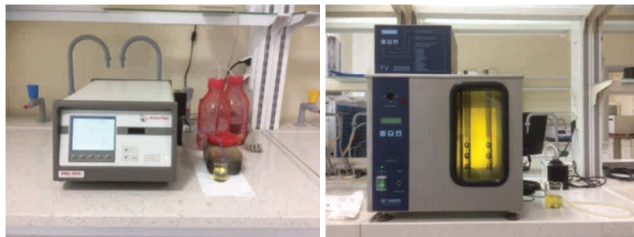
Fig. 3. DMA 4500/5000 for density determination and TV 2000 viscometer for determining kinematic viscosity
