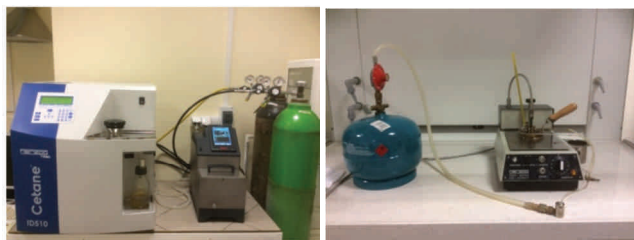
Fig. 4. Cetane ID 510 for determining a cetane number and Device for determining the flash point
