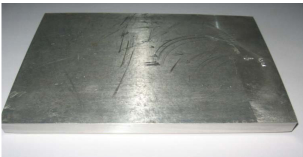
Figure 3. Al - austenitic CrNi steel bimetal
