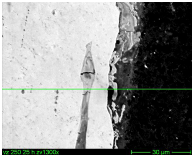
Figure 5. Concentration line profile using EDX analysis
