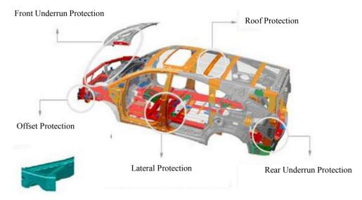
Fig. 1. The safety features of the vehicle structure [1
