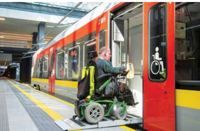
Lifts for passengers on wheelchairs Source: ŁKA.
