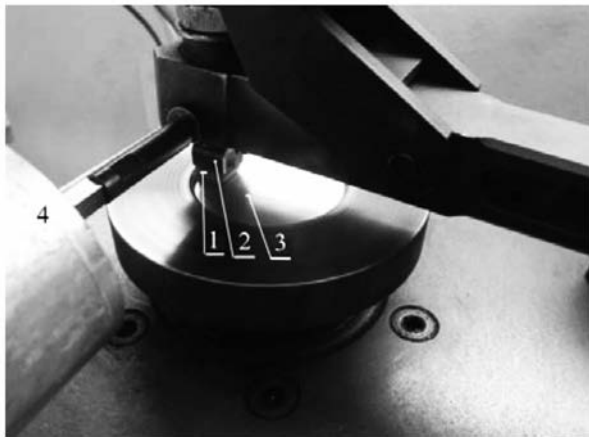
Fig. 4. Friction contact of T-01M tester: 1 – sample, 2 – sample holder, 3 – countersample, 4 – friction force gauge
