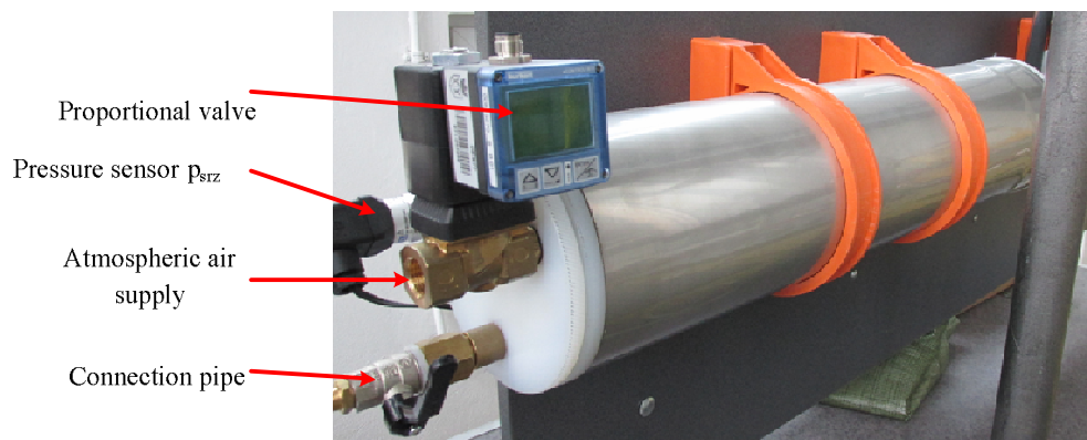
Figure 3. Container of suction pressure which supplies milking machine
