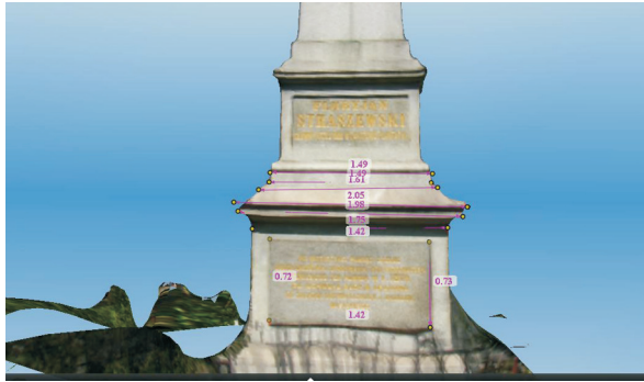
Fig. 5. Examples of measurements on the monument model generated from long-series images
