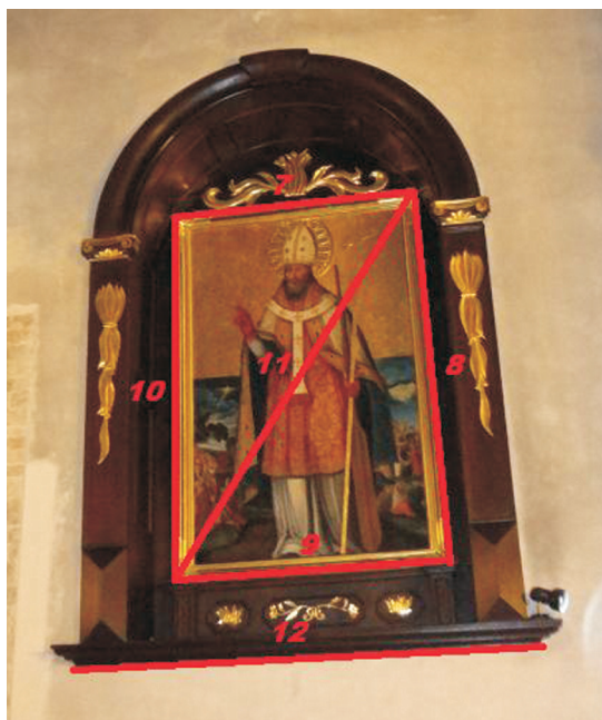
Fig. 8. Selected elements of the model were compared with the direct measurement (7–12)
