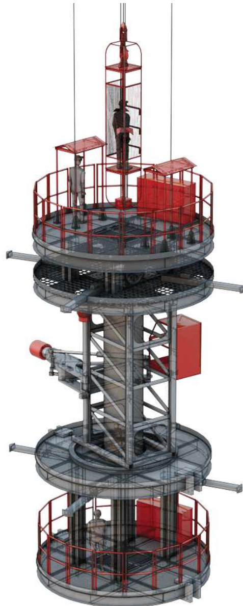
Fig. 2. A view of the shaft reaming machine
