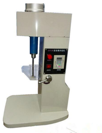
Fig. 2. View of XFG laboratory flotation cell
