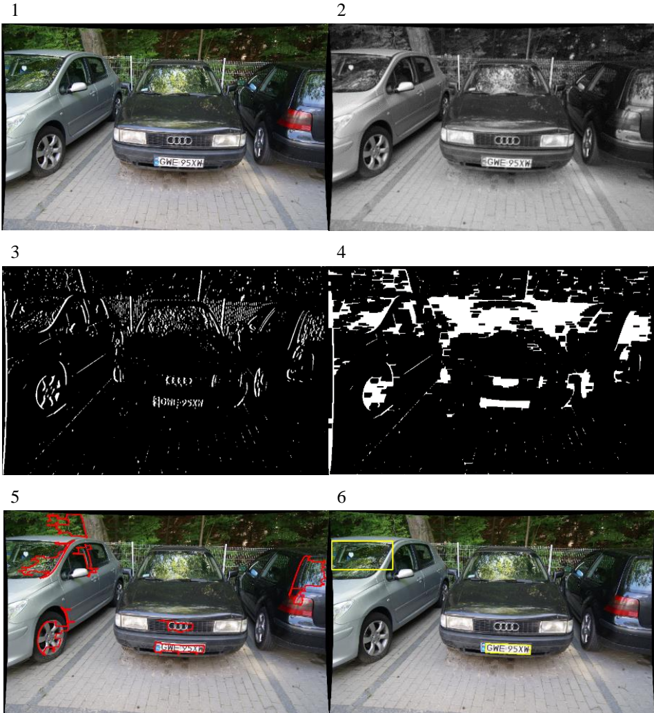
Fig. 3. Results of image segmentation: 1 — original image, 2 — bit image, 3 — Sobel transformation, 4 — picture after morphological operation, 5 — detected contours, 6 — validated tiles prepared to SVM classification
