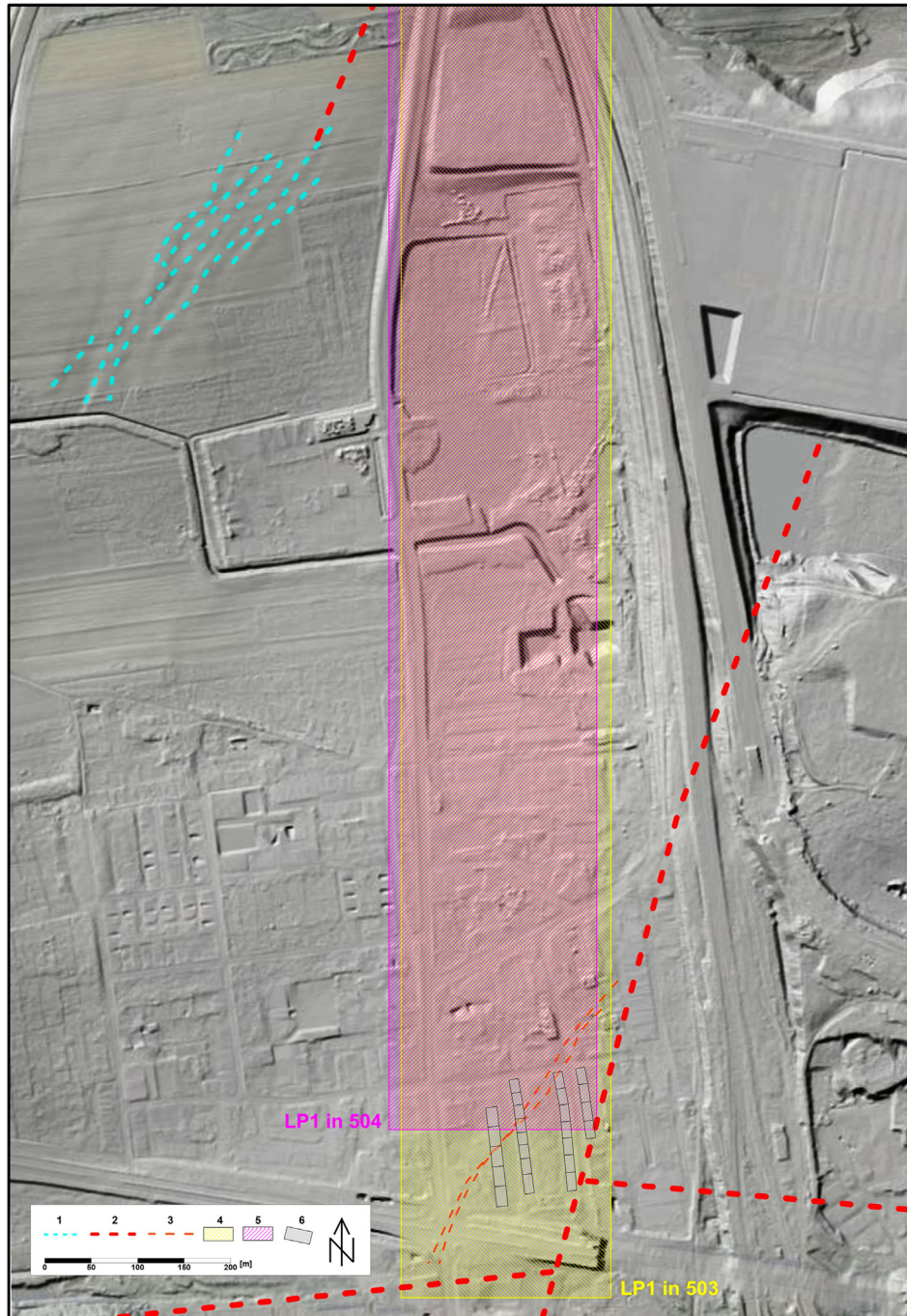
Fig. 6. Lineaments in the region of one of the Triassic fault visible in the hillshade image of the numerical relief model [28] after extraction of coal by the LP1 longwalls in 503 and 504 seams. 1 – lineaments, 2 – tectonic faults in Triassic, 3 – tectonic faults in 503 and 504 coal seams, 4 – panel LP1 in 503 seam, 5 – panel LP1 in 504 seam, 6 – damaged building segments.
