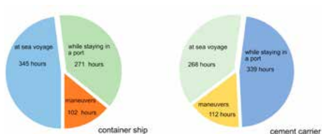
Fig. 1. Total times of operating states of a container ship and a cement carrier realized in one month [own source].
