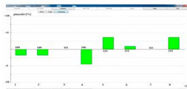
Fig. 2. Deviations from the mean value of the combustion pressure at the beginning of the first stage of the engine start-up.
