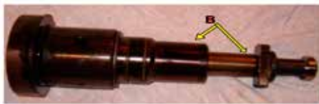
Fig. 18. Local traces of scuffing on the barrel/plunger injection pump.
