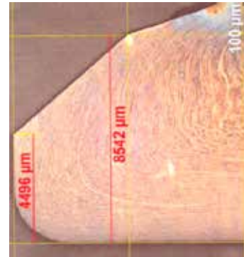
Fig. 11. Valve thickness measurement in the faying section.
