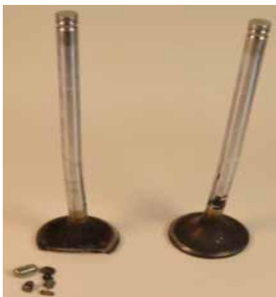
Fig. 5. View of studied damaged valves.
