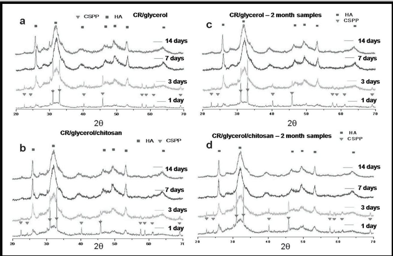
FIG. 2. The X-ray diffraction spectrum of the (a) R cement/glycerol and R cement/glycerol/chitosan (b) samples after different times (1, 3, 7 and 14 days) of immersion in Ringer's solution. (a-b) time-zero samples, (b-c) samples after two month of storage in the freezer.
