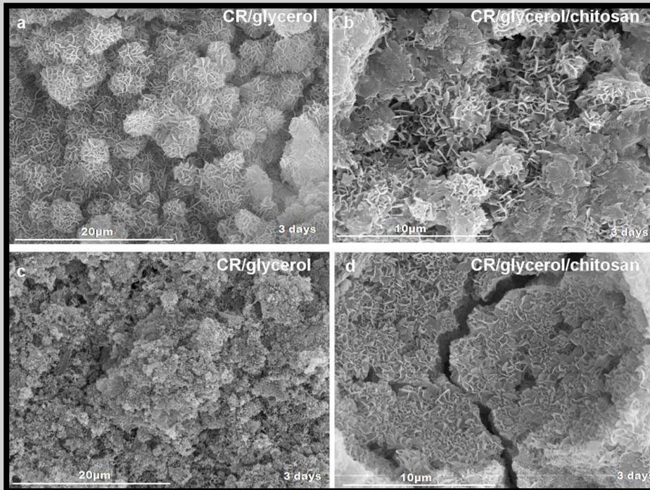
**FIG. 4.** SEM micrographs of R cement scaffold: (a-b) time zero samples; (c-d) two-month samples.
