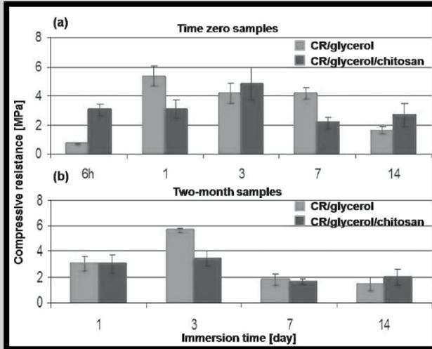
**FIG. 3.** Mechanical properties of (a) time zero samples after different times (6h, 1, 3, 7 and 14 days) of immersion in Ringer's solution and (b) samples after two-month of storage in the freezer.
