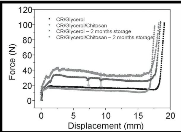
FIG. 1. Injection force vs. syringe displacement for R-cement and R-cement/chitosan pastes before and after storage in the freezer.
