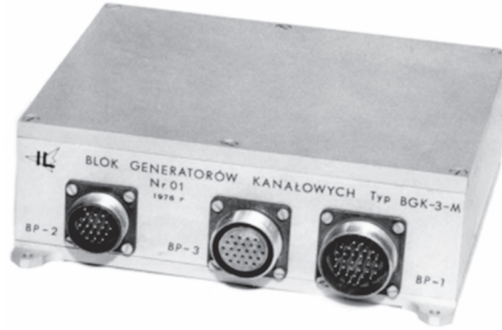
Fig. 1. Block of channel generators BGK-3-J (M), designed for Intercosmos -15, 18, 19 programmes (1976-79), [7]
