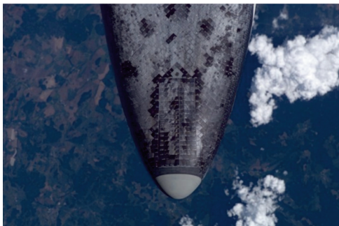
Fig. 4. Heat shield tiles as an advanced flexible reusable Surface insulation and thermal insulation composed of multiple layers of thin sheets [15], [16]
