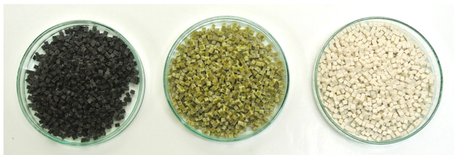
Figure 4. View of granulated propellants: (a) modified No. 2, (b) Szmaragd/Szafir (Sz/Sz), (c) modified No. 1
