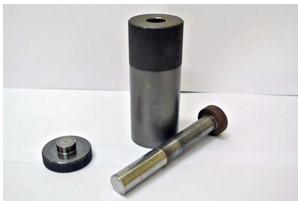
Figure 5. View of the die for propellant pressing (23 mm diameter)
