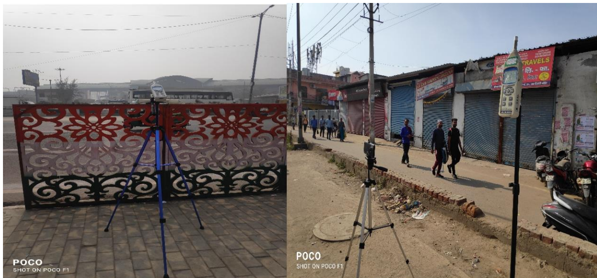
Fig. 3. Image showing SLM and camera installed at site
