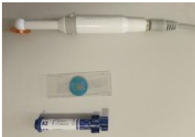
Fig. 5. Silicone mold filled with composite
