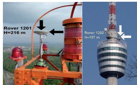
Fig. 11. Positions of two receivers on the TV tower at different levels above ground
