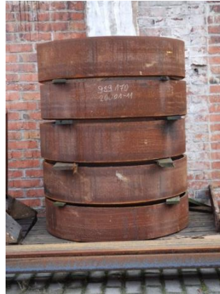
Fig. 1. Specimens pipes with a diameter of 914.4 mm (36"), wall thickness of 17.1 mm and 250 mm in length, API 5L X70 steel
