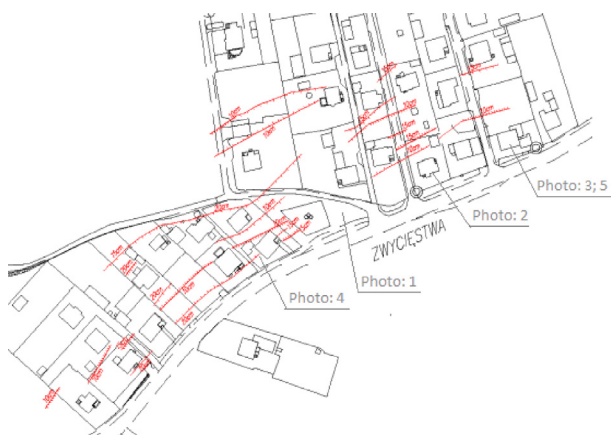
Fig. 3. Sketch of the LDGD with the heights of the steps and the structures made up of them.
