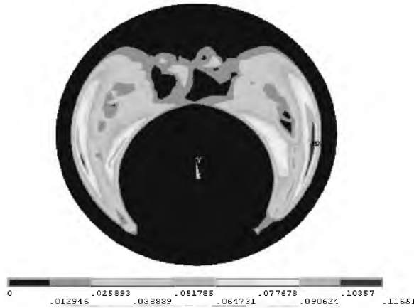
Fig. 6. Fluid velocity in exemplary cable conduit
