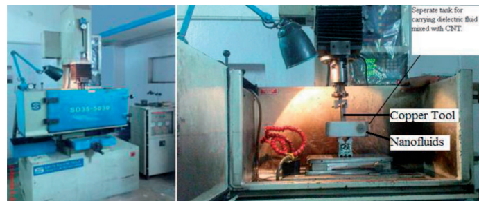
Fig. 2. EDM machine with nanofluids and electrode setup
