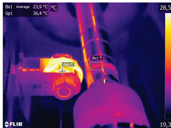
Fig. 7. Measurement of burnisher and workpiece temperature (test no. 1)
