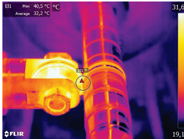
Fig. 5. Area of measuring the temperature of tool-workpiece contact
