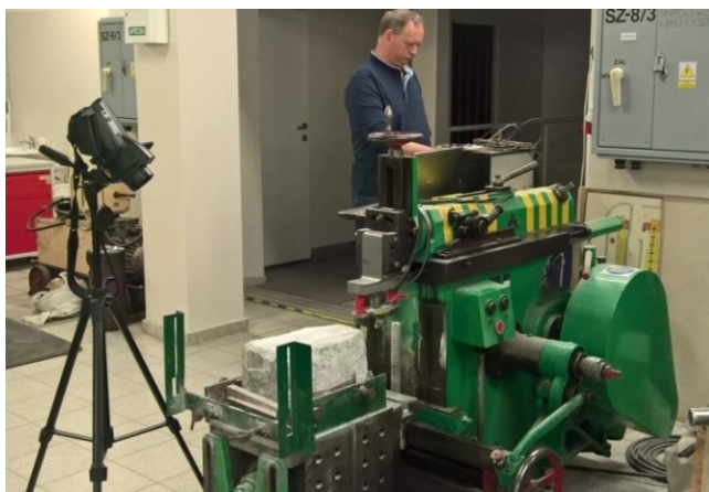
Fig. 11 Shaper-based cutting resistance test stand with a strain-gauge head
