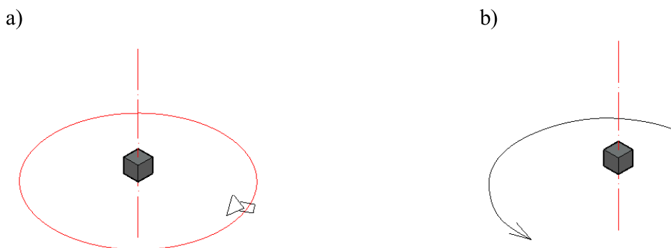
Figure 3: Creation an object panorama by: a) a camera rotation, b) an object rotation
