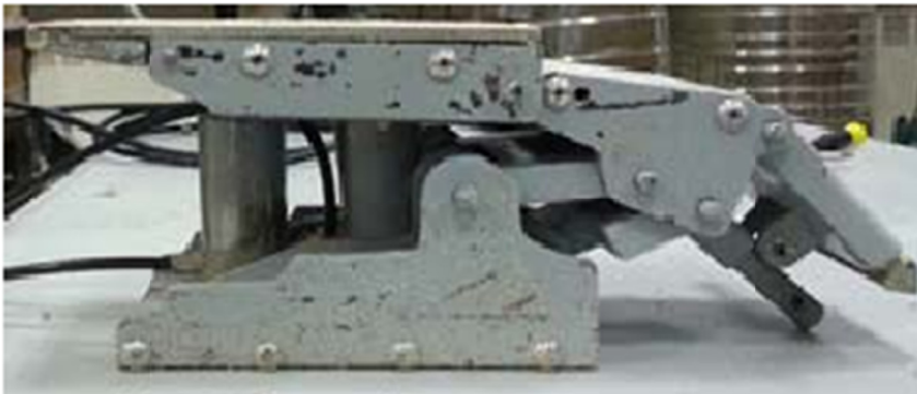
Fig. 5. Hydraulic support used in the experiment
