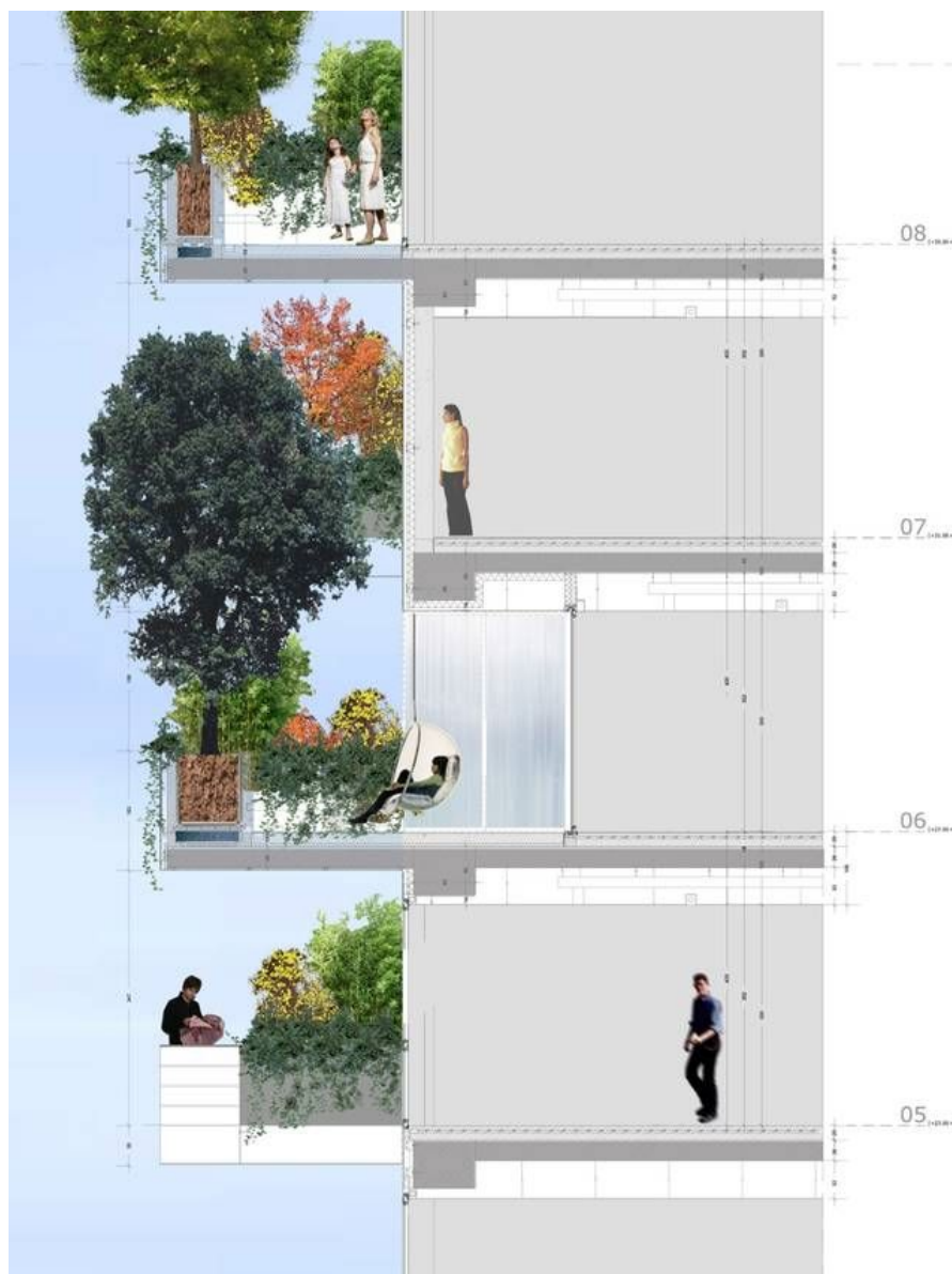
Fig. 4. Front wall cross section, Nanjing Vertical Forest, Nanjing, China, arch. Stefano Boeri Architetti. Source: Stefano Boeri Architetti, http://media.treehugger.com/assets/images/2013/03/vertical-garden.jpg.650x0_q70_crop-smart.jpg [access: 10.03.2017]. Ryc. 4. Przekrój ciany frontowej budynku Nanjing Vertical Forest, Nanjing, Chiny, proj. Stefano Boeri Architetti. [dost p: 10.03.2017].
