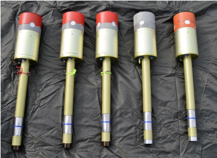
Fig. 3. Interception net deployment projectiles ready for use
