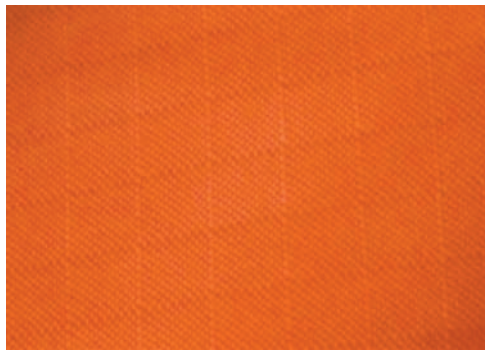
Figure 4. F-111 nylon fabric with a distinctive ripstop weave usually used in parachute canopies (HORNET).
