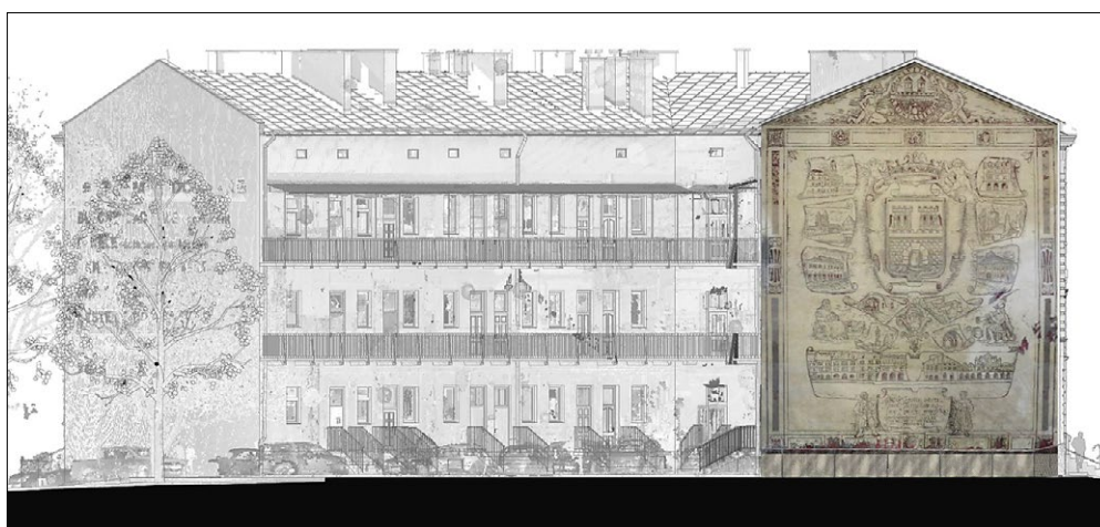
Fig. 2. Elevation view with sgraffito mapped using photogrammetry, against the background of a snapshot view of a model with a point cloud as a base; by the authors.
