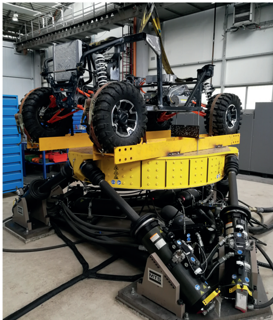
Fig. 2. Platform construction during the test at the M.A.S.T. stand
