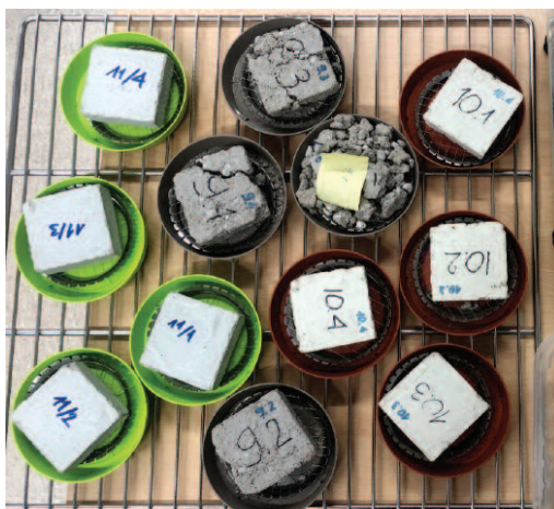
Photo 4. Some of plaster samples after sorption tests – destruction of series 9 samples is visible
