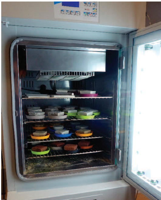
Photo 1. Plaster samples for sorption tests in climate chamber
