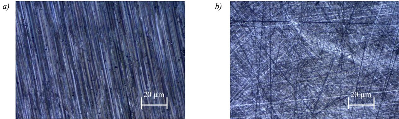
*Fig. 1. Workpiece surface of steel C45: a) after grinding, b) after lapping with SiC-F400,  $p = 0.04$  MPa,  $v = 49$  m/min*
