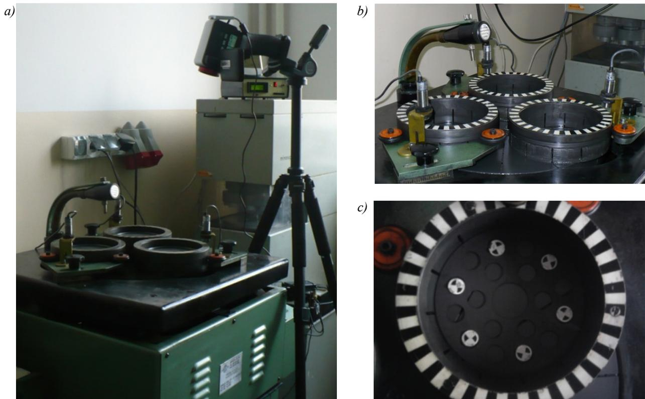
*Fig. 5. Experimental setup: a) general view, b) executory system, c) samples condition in conditioning rings*
