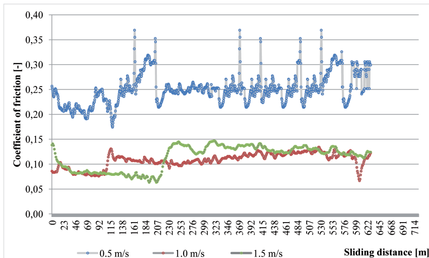
Fig. 6. Coefficient of friction for tests with POE lubricant (series 4–6) with load 120 N
