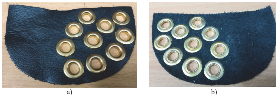
Fig. 10. The natural leather with the installed grommets in a dynamic mode: a) inner side, b) outer side
