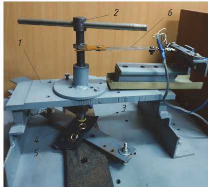
Fig. 4. The device for performing the operation of metal fittings installation: 1 – holster; 2 – a pair of screws for loading; 3 – material with the grommet; 4 – working tools (punch and matrix); 5 – strain gauge for measuring the installation effort; 6 – strain gauge for measuring the value of the punch movement
