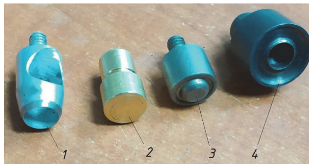
Fig. 1. Working tools: 1 – punch; 2 – punch-cutting board; 3 – punch; 4 – matrix
