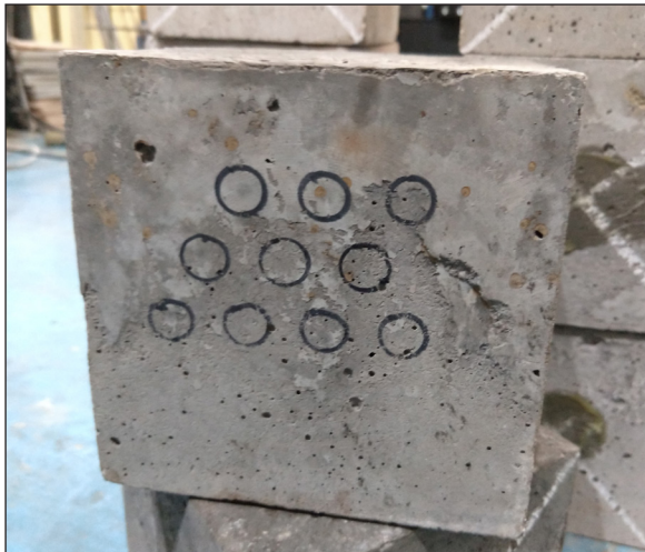
Fig. 2. Rebound Hammer test locations
