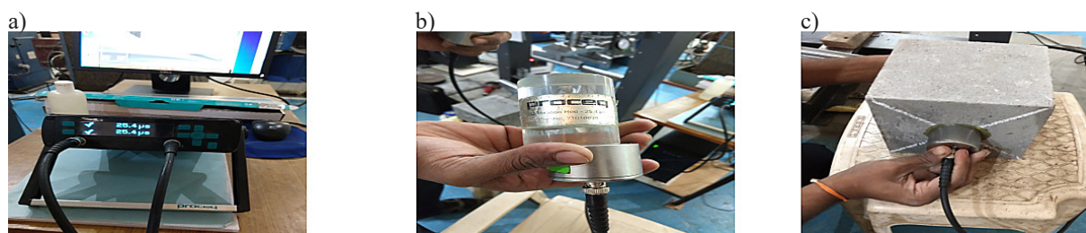
Fig. 4. Ultrasonic Pulse Velocity Test procedure; a) UPV machine, b) Calibration sample, c) UPV measurement
