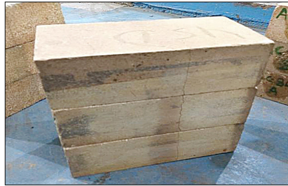
Fig. 18. Sample B-2 cracked after 6 cycles
