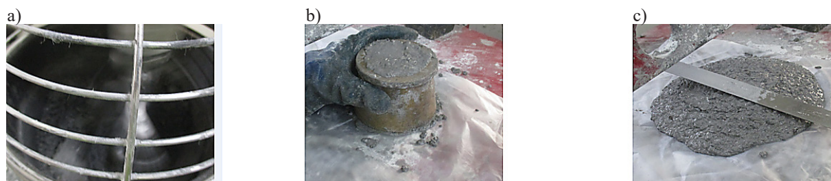
Fig. 1. Fresh 80% Al 2 O 3 concrete test cubes preparation; a) Hobart Mixer, b) Slump cone test, c) Consistency test
