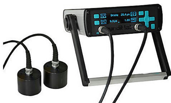
Fig. 5. Graphical illustration of UPV Test
