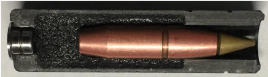
Fig. 3. Cross section of 6.8 mm CT cartridge (www.gatdaily.com)
