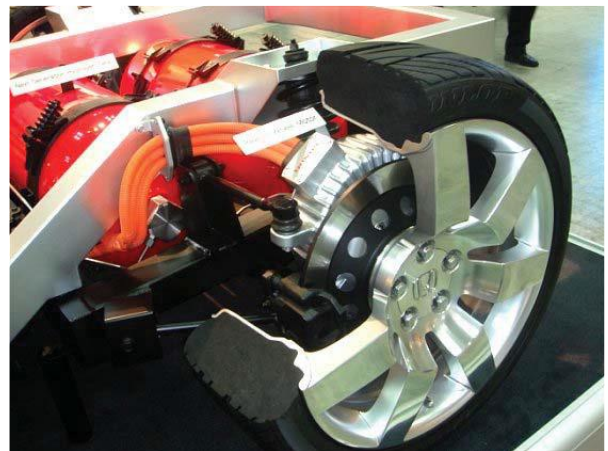
Fig. 9. Direct drive system designed by Honda [8]
