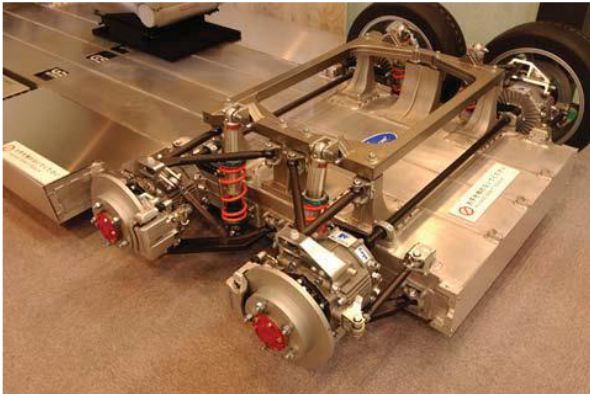
Fig. 7. High-speed motors arranged in the Japanese car test Ellica [6]
