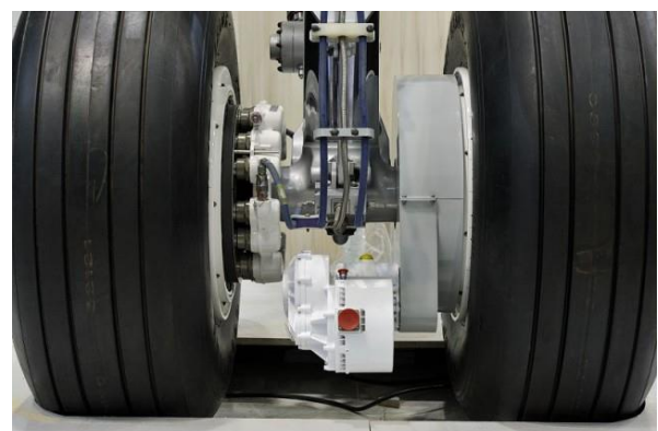
Fig. 3. The EGTS 50 kw motor and drive system on the A320 main gear. It's the white and grey unit. [3]
