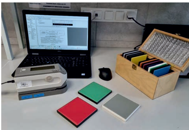
Fig. 3. Test stand for determining colour according to EN ISO 7724-2 [22]; Konica Minolta CM2600D spectrophotometer, CCSII Lucideon Ltd spectrophotometric standards [Pic. M. Garbacz]
