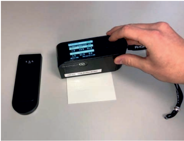
Fig. 4. Test stand for determining gloss in accordance with EN ISO 2813 [24]; Rhopoint IQ-S glossmeter [Pic. M. Garbacz]
