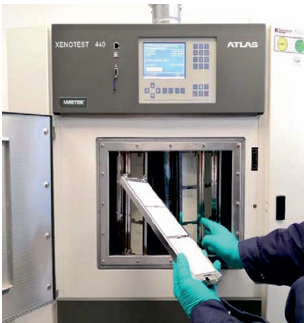
Fig. 2. Test stand for ageing samples according to EN 16474-2 [11]; xenon weathering instrument, Atlas GmbH Xenotest 440 [Pic. M. Garbacz]
