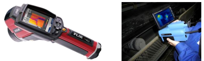
Fig. 2. Thermal imaging camera FLIP i40, and Therma Cam PM 454 during measurements on conveyor belts (SKF)
