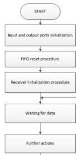
Fig. 7. Process of initializing modules in the receiver state [7]
