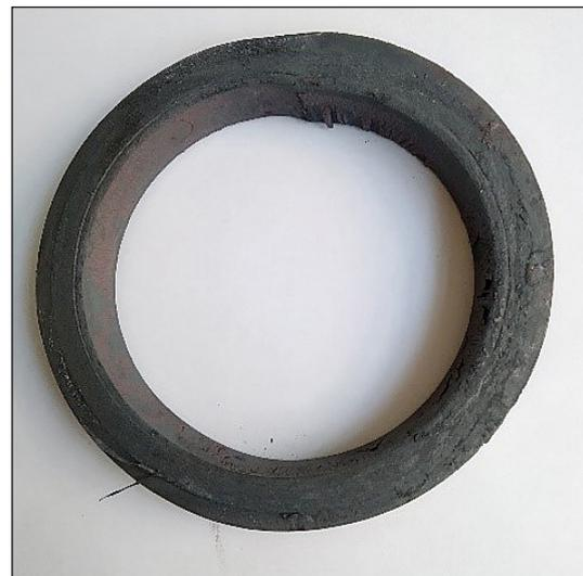
**Fig. 8.** Ring with a defect, as formed in the rolling process conducted with a feed speed of 40 mm/rev
