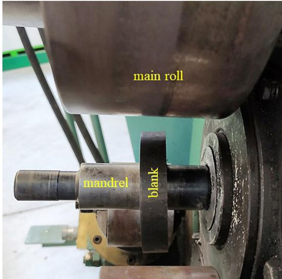
**Fig. 3.** Schematic (a) and real view (b) of the radial ring rolling process
