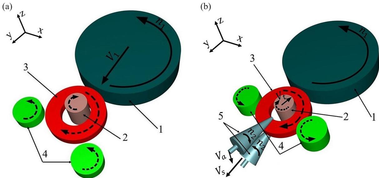
**Fig. 1.** Schematic representation of the ring rolling process: (a) radial ring rolling, (b) radial-axial ring rolling; 1 – main roll, 2 – mandrel, 3 – ring, 4 – conical rolls, 5 – calibrating rolls
