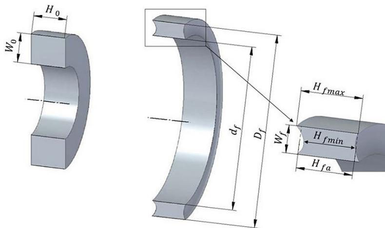
**Fig. 4.** Schematic of the ring cross-section before (a) and after (b) the rolling process;  $W_0$  – initial width of the ring,  $H_0$  – initial height of the ring,  $H_f$  – final height of the ring,  $H_{fmax}$  – final maximum height of the ring,  $H_{fmin}$  – final minimum height of the ring,  $H_{fa}$  – final average height of the ring
