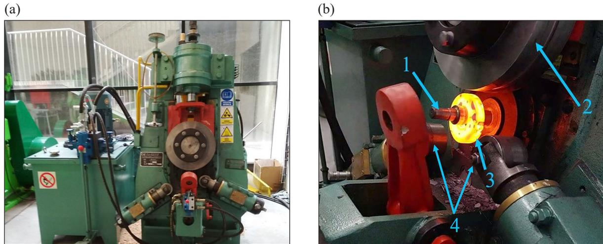
Fig. 2. D51Y-160E rolling mill used in experiments (a) and the initial stage of the rolling process conducted with the following tools (b); 1 – mandrel, 2 – main roll, 3 – ring, 4 – calibrating rolls
