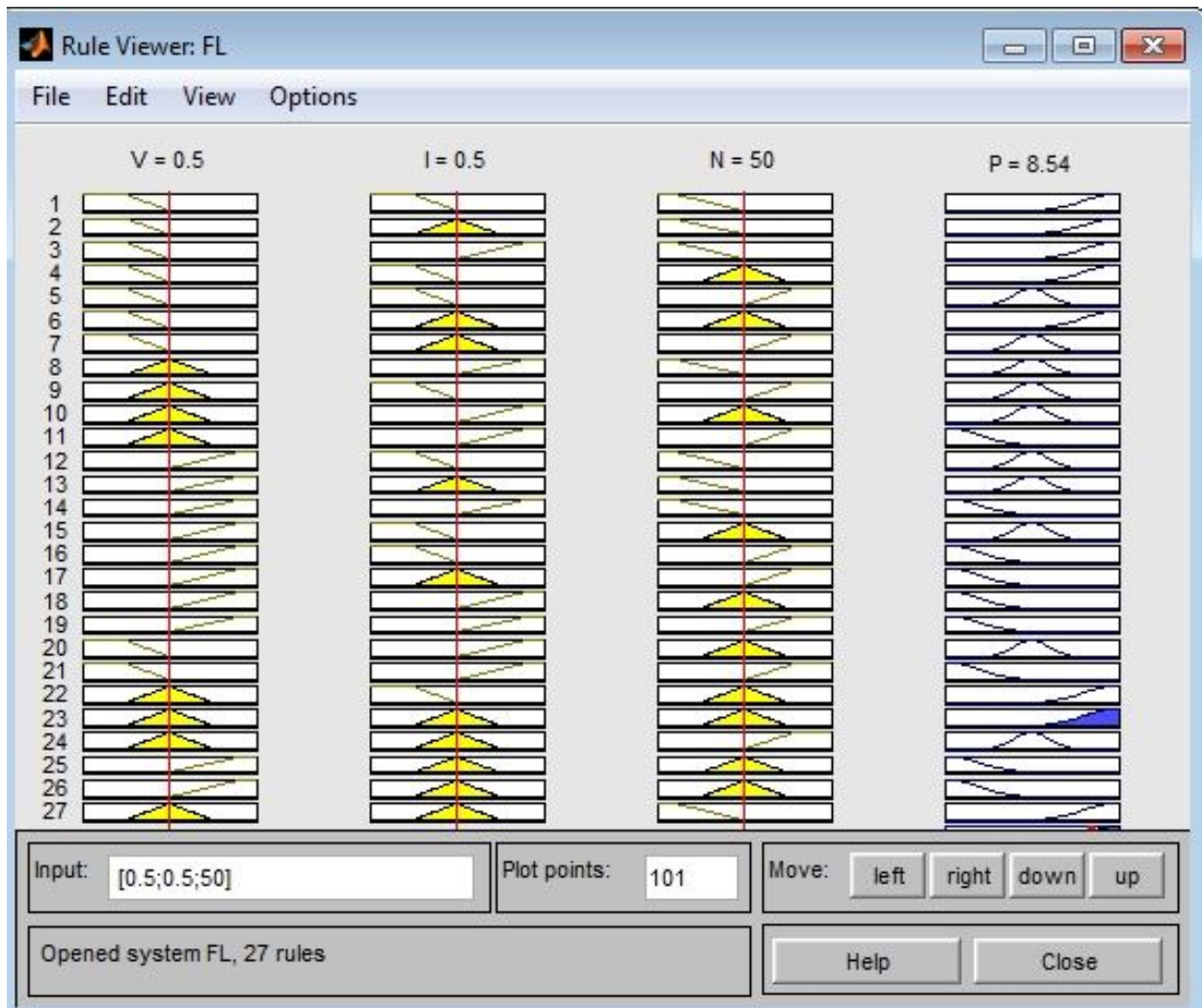
Fig. 2. View window of the rules of fuzzy inferences in MATLAB software environment
