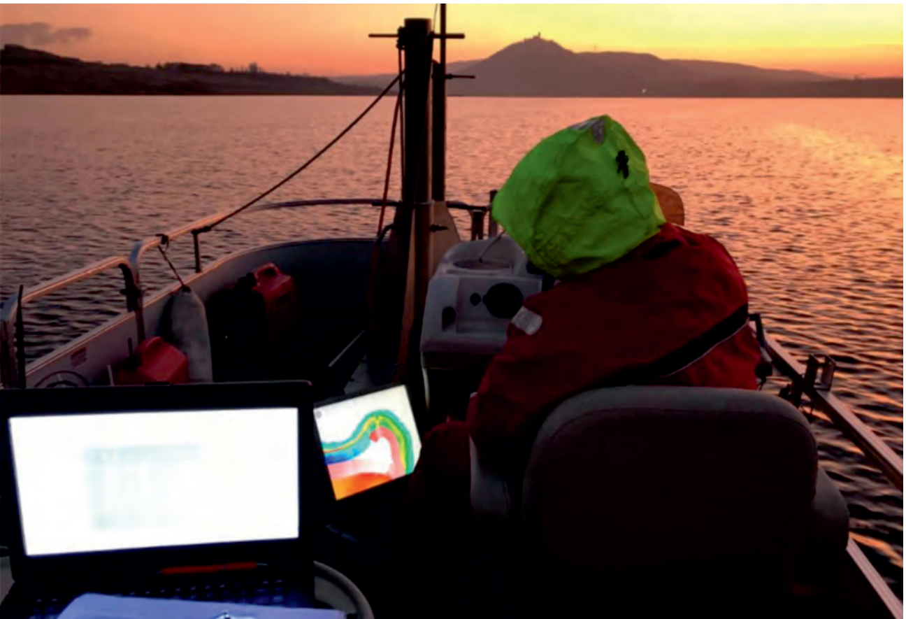
Rys. 9. Pomiary batymetryczne na zbiorniku Most [6] Fig. 9. Bathymetric measurements on Most reservoir [6]
