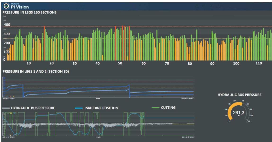
Fig. 7. Current view of pressures in powered support sections
