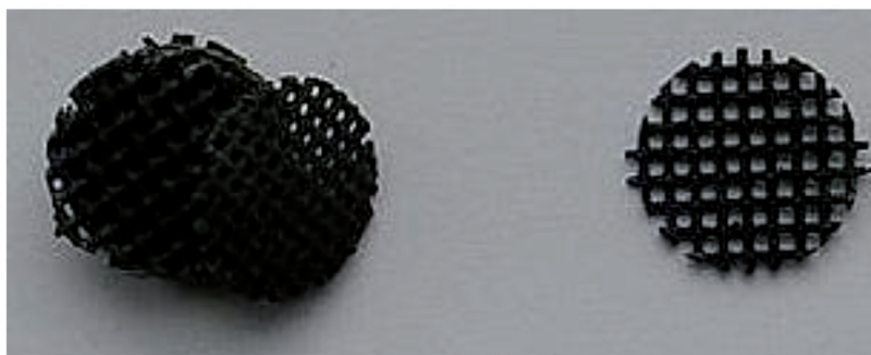
Fig. 1. Platinum catalyst supported on steel-ceramic wire mesh, manufactured by Catator [Author, 2014]
